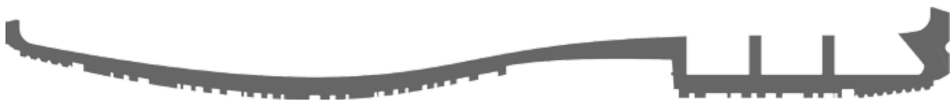
Outsole cross-section | Cleatdepth 2,7 mm | Effective thickness 4,0 mm
