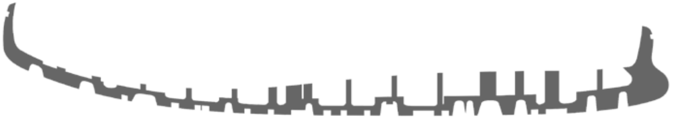
Outsole cross-section | Cleatdepth 4,0 – 3,0 mm | Effective thickness 1,5 mm
